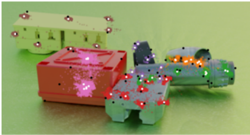
Figure 4.11.: Keypoint proposals and final predictions of the standard FFB6D network on a sample from the SCAPE 2 test set. Predicted keypoints are colored in white. The ground truth keypoints are colored in black. The keypoint proposals for each object are in a separate color.
